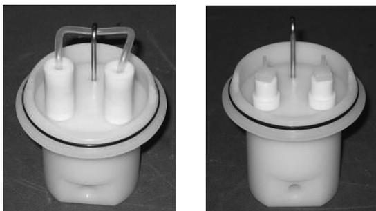
**Note:** Ensure the reagent bottle adapter connectors (2100RF) are finger tight to prevent possible leakage of sample into the reagent.
