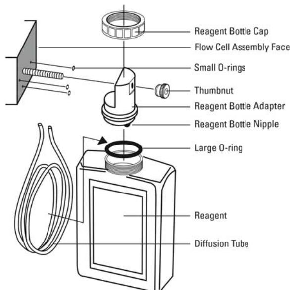
Figure 14: Reagent Bottle Assembly
