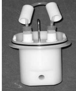
5. Press the diffusion tubing assembly caps onto the adaptors and loop the tubing onto the hook, as shown in the figure below.
