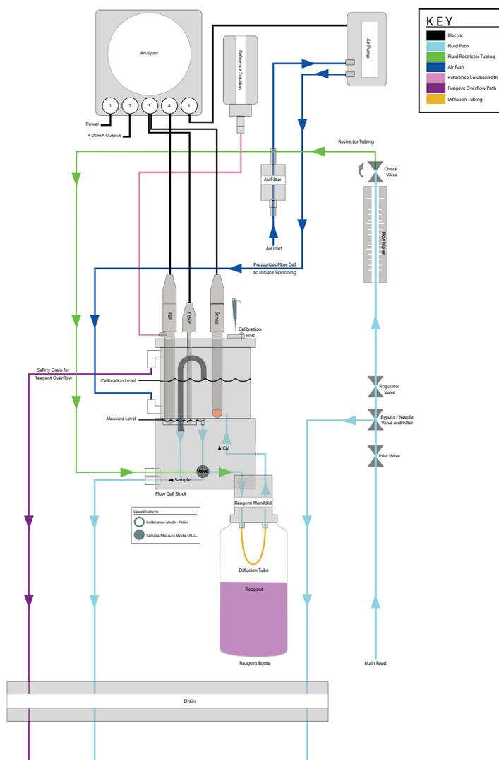
The sensing electrode responds logarithmically to changes in the sodium ion concentration. This response is described by the Nernst equation:
