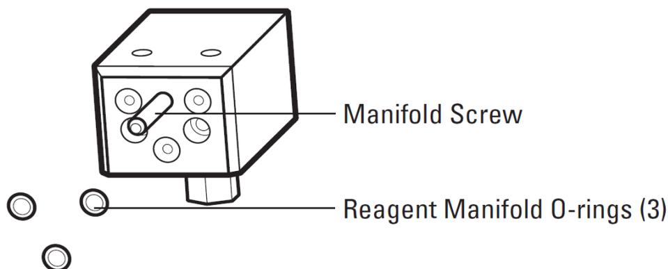
Figure 26: Reagent Manifold O-ring Location
