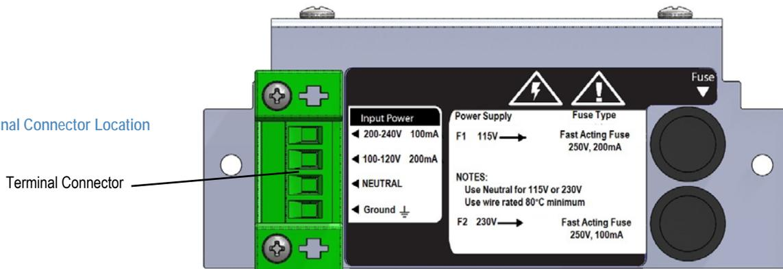
4. Feed the power cable through the conduit or cable glands as required.
