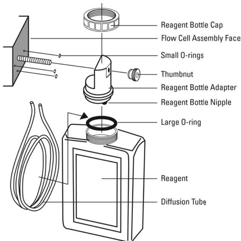
Figure 27: Reagent Bottle Assembly
