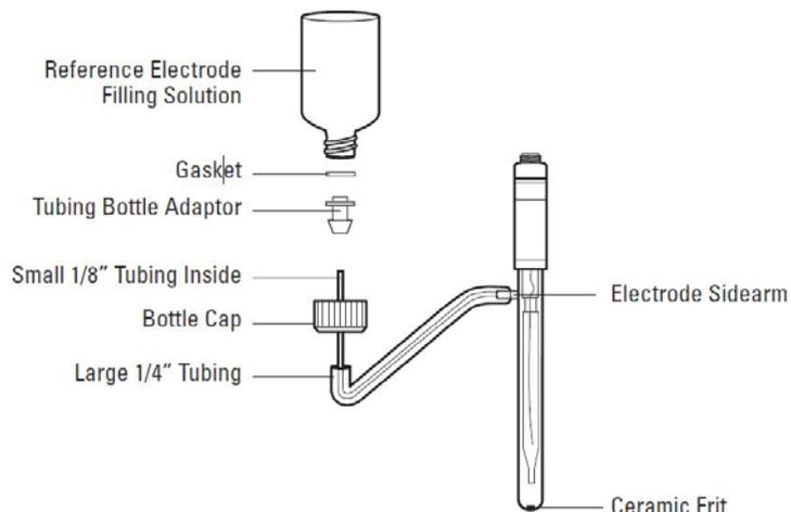
8. Invert the electrolyte bottle and snap it into the clip. Refer to Figure 18. Use the pushpin supplied with the reference electrode to puncture three air vents on the bottom of the filling solution bottle.
