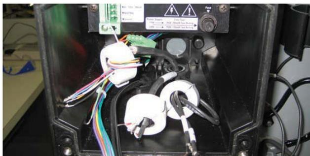
Figure 15: Ferrite Installation
