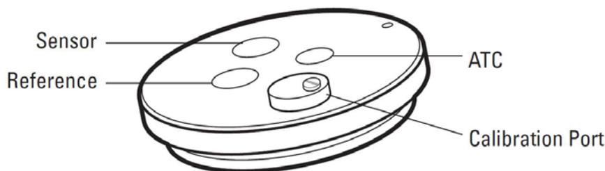
5. Plug the electrode cable marked "Sensing" into the top of the electrode. Be sure to push back the black cap to verify a secure connection between the male and female pin connection prior to tightening.
